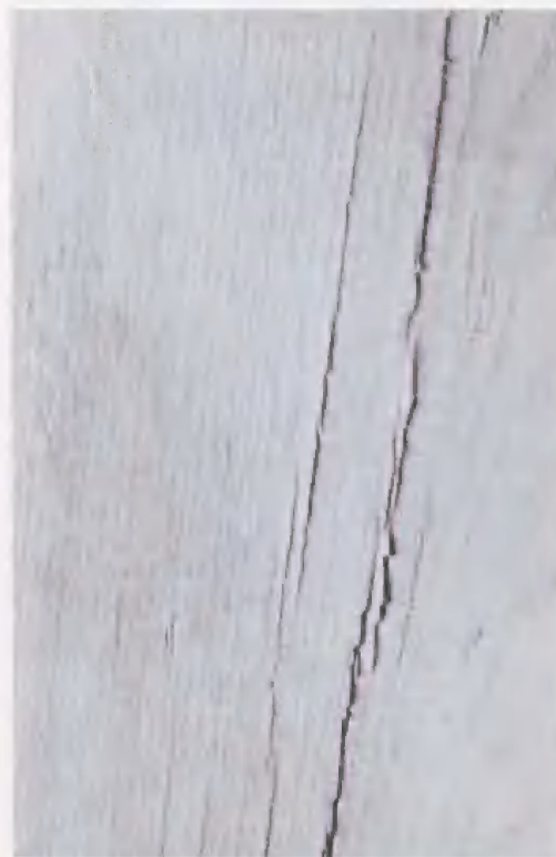
Shake: Occurs lengthwise between or through the growth ring.
